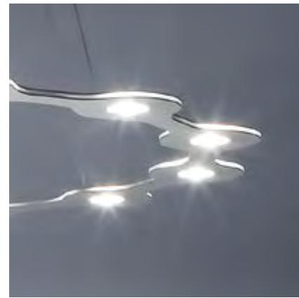
Series of slender suspension lamps with 3, 6, or 12 LED light spots arranged in a circle. The structure is 8 mm thick and made with two sheets of natural anodized aluminum interposed by a layer of transparent methacrylate. It creates indirect light upward and direct light downward through polycarbonate lenticular diffusers. A variety of finishes are available. Includes dimmable power supply embedded in the ceiling rose and self-supporting transparent power cables.
